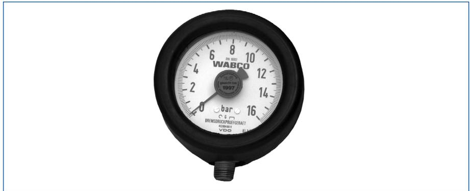
Shown in the image is test pressure gauge 453 004 007 0 ending at 16 bar on the dial. The marking line indicating the permitted deviation of the pointer position in a steady position is across from the 0 mark. Next to it is the position symbol which needs to be noted when using the instrument.
