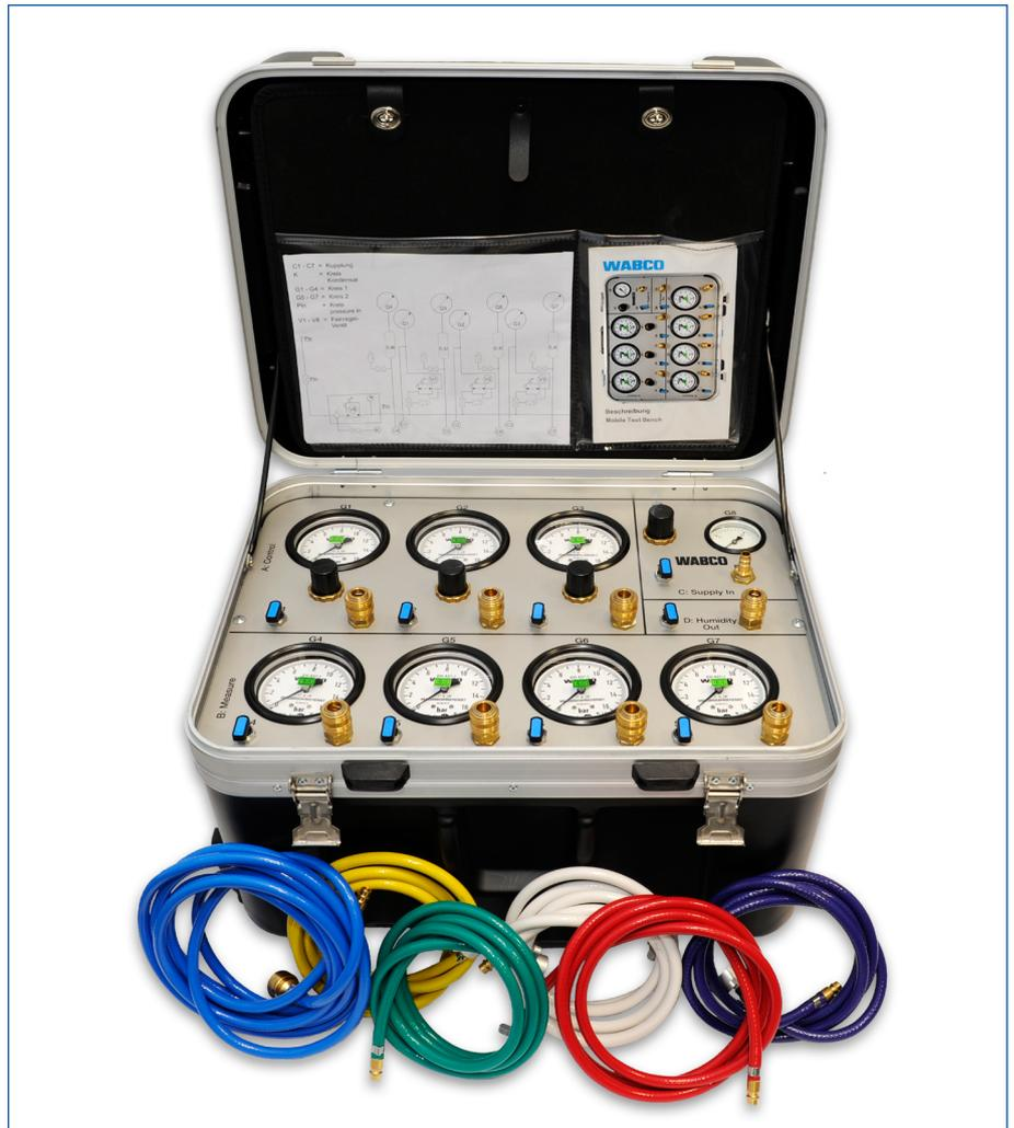
The mobile test bench has been devised as a get-started tool for garages which inspect and service braking devices.
