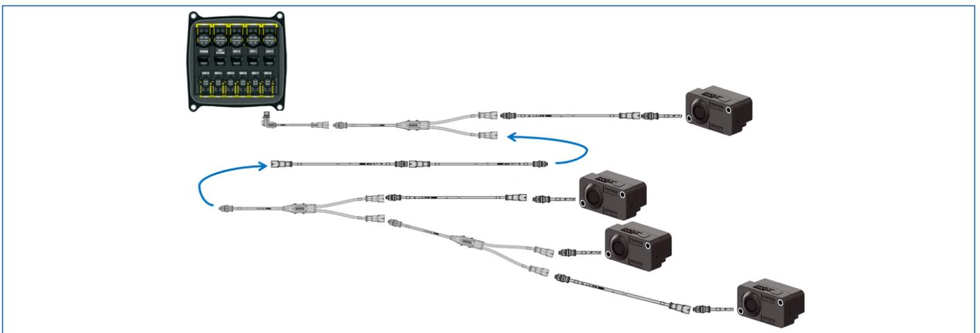
The ultrasonic sensors transmit ultrasonic waves to the area behind the vehicle. If an object or a person reflects these sonic waves, the ultrasonic sensors receive an echo. The distance to the object is calculated from the time the ultrasonic waves take from transmission to reception of the echo.
