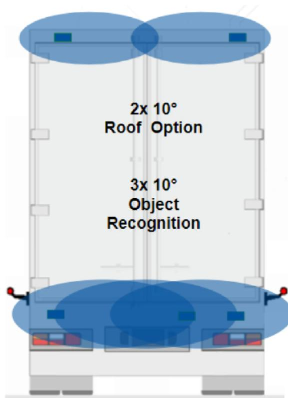
Sensors are installed horizontally at a height of at least 60 cm. The viewing direction of the sensor membrane is always aligned with the centre of the back of the vehicle.
